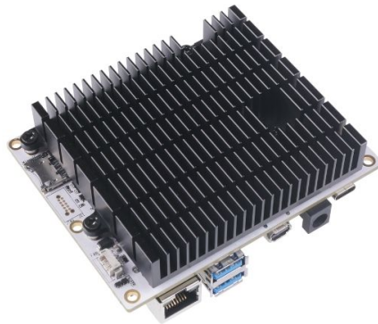
Fig. 6.10: BeagleBone AI-64 back with heatsink at 45° angle
